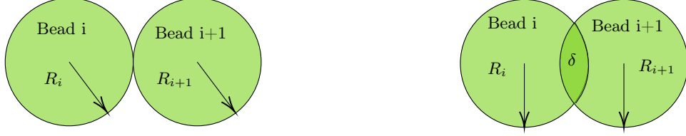
Figure 2: Hertzian contact and deformation of the granules. It represents the deformation of the granules at the contact point.
