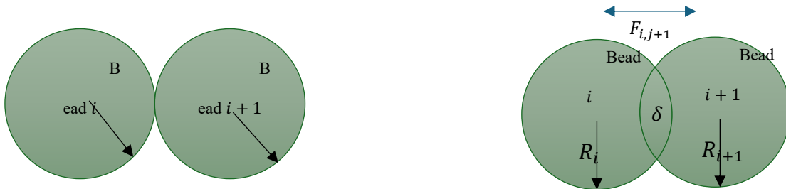
Figure 3: Hertzian contact and deformation of the granules. It represents the deformation of the granules at the contact point.
