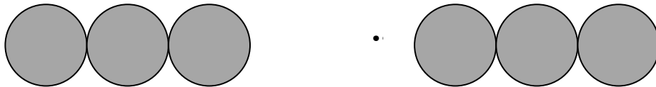
Figure 2: Hertzian Contacting Granules. A series of Granules are connected in a series and the repelling force ( F ) varies nonlinearity with deformation \delta .
